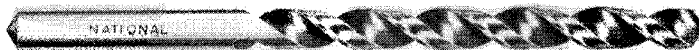
Figure 4-9 High-helix drill designed with higher cutting rake and improved chip conveying properties for use on materials such as aluminum, die-casting alloys, and some plastics. (Courtesy National Drill and Tool Co.)
